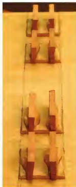
Last step. Add glue and tap in the wedges. After the glue dries, saw the wedges flush.
